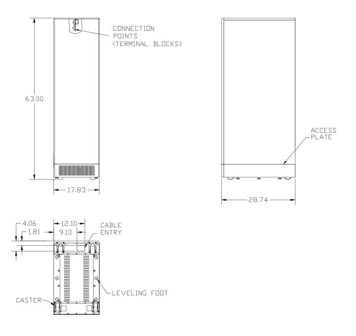
Figure 12 – "E" Battery Cabinet Drawing for 50/80kVA Ratings
